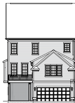
REAR ATTACHED GARAGE ELEVATION DETAIL
